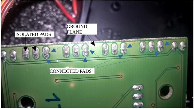
You can verify this by continuity testing (with a Multimeter)
